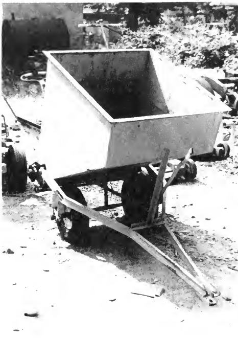
A small sander for small jobs. It could be towed behind even a small lawnmower-type tractor, or pushed by hand.
